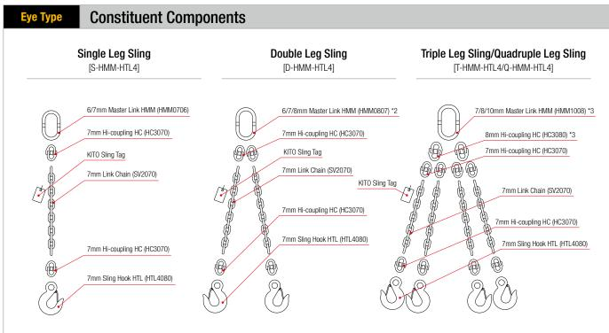
•For single leg slings, use components that are appropriate for the W.L.L. (Working Load Limit) of the link chain that is used.
